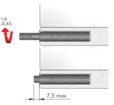
WITH MAGNET for cabinets using unsprung hinges or negative hinges.
