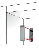
ANTI-TURNOVER LOCKING Stop screwing the red bolt when it touches the wall plate
