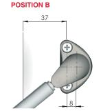
The opening of the door can be changed by adjusting the position of the side bracket:
