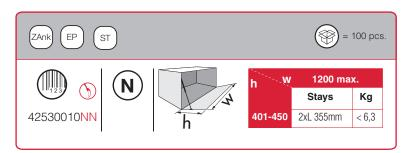
This chart refers to chipboard or MDF 18 mm doors and aluminium frame doors with glass 4 mm thick using standard, flap or Kimana hinges. These are experimental results to be checked by the customer. For a better function and for safety reasons, we suggest to use at least two stays per piece of furniture (extra-size doors might require 3 or more gas stays). For doors whose weights/dimensions are bigger than those reported on the chart, please increase the number of stays accordingly.
