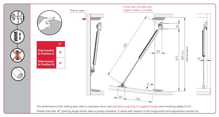
For pistons quantity to be specified according to door size, refer to the chart for "COMPACT 355 mm - DROP DOWN".
