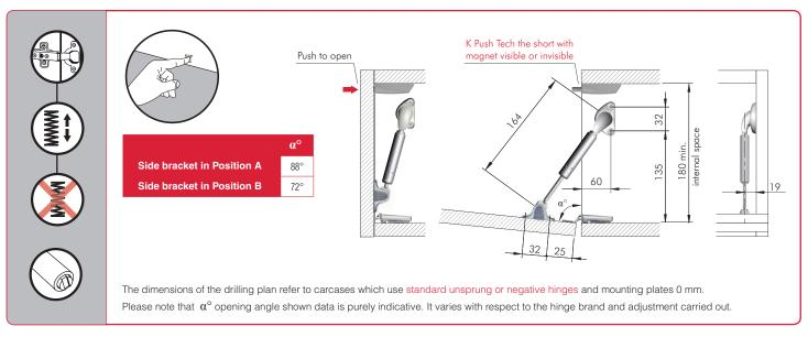
For pistons quantity to be specified according to door size, refer to the chart for "COMPACT 164 mm - DROP DOWN".
