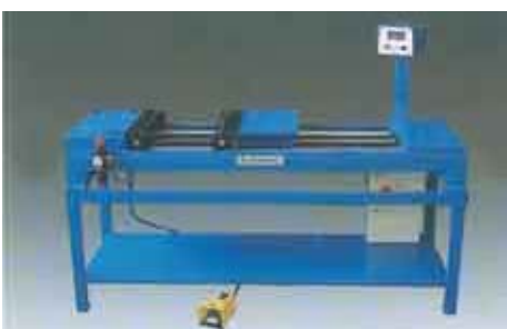
FAST 3 / FAST 4 Pneumatic bending machine for drawer mass production. E. Patent: 0 674 968 U.S. Patent: 5.535.504
