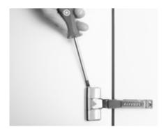
Use a screwdriver (PZ2) to adjust the damping effect (- 20% by two steps).
